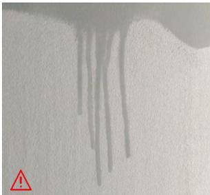
It absorbs water quickly, like a blotter. Excessive penetration of adhesive / Lack of slip / Poor bonding.
