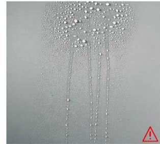
The water runs off and beads on the wall.
