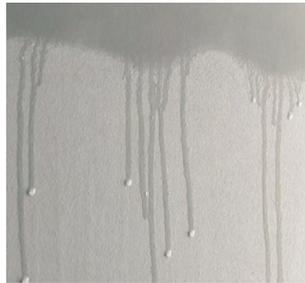
The water runs off, leaving a wet trail that is absorbed in under 2 minutes
